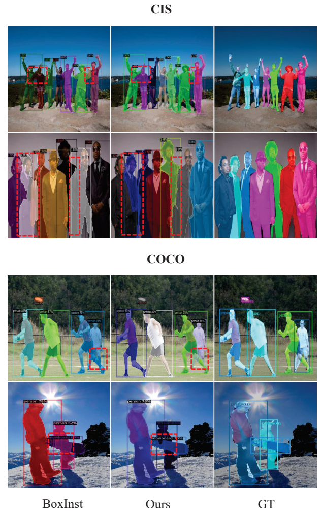
Fig. 4. Visualization of instance segmentation on CIS and COCO. As shown in red dash boxes the proposed OverlapLoss can generate higher quality instance segmentation.
